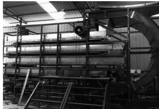
图8 麦冬热风循环箱式干燥、揉搓、去须一体机 Fig. 8 Ophiopogon hot air circulation box type drying, kneading and shaving machine of Ophiopogonis Radix
