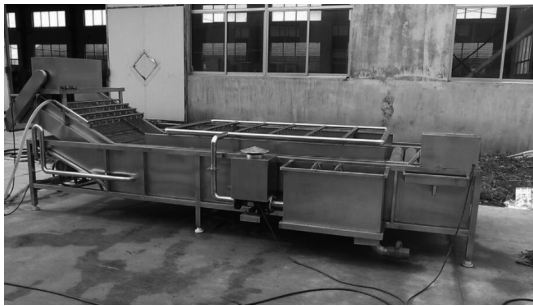
图6 根茎类中药材通用超声波清洗机 Fig. 6 Universal ultrasonic cleaning machine for root and stem Chinese medicinal materials
